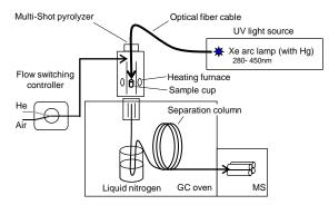
Fig. 1 UV/Py-GC/MS system configuration
